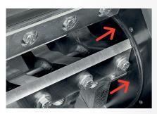
Rotary discs integral with the rotor and containment rings. Bench adjustment of rotating and fixed knives.
