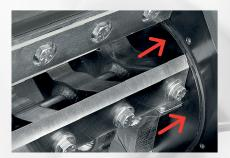
Rotary discs integral with the rotor and containment rings; bench adjustment of rotating and fixed knives. Scissors cutting configuration.
