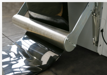
New redesigned pneumatic dancing arm that guarantees the process of every type of sheet from full sheet to full sheet with cups still attached.
