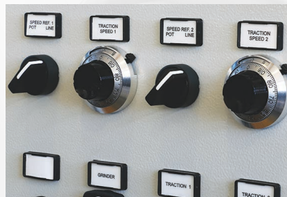
Edge trims feeding speed adjustment by inverter, synchronized with the extrusion line.
