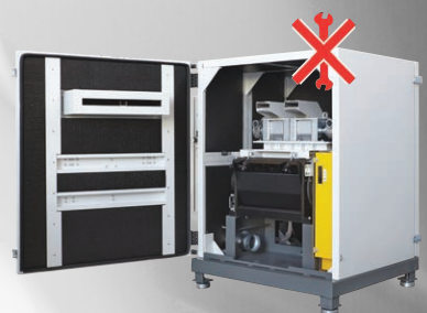
Easy access from one side only to all the parts interested for ordinary maintenance.
