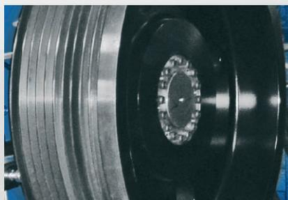
Keys for the fixing of motor pulley and flywheel. Pulley and flywheel manufactured as per drawing due to high inertia.
