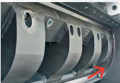
Rotary discs integral with the rotor and containment rings.
