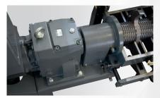
Gearmotor aligned with the rotor by interposed chain joint.
