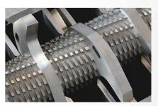
Gradual cut and reduced cutting stress to the minimum thanks to the helical toothed rollers.
