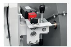
Rotor lock for maintenance. Safety devices and circuit in compliance with EEC Directives.
