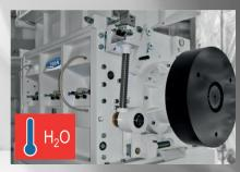
Water cooling system of the grinding chamber.
