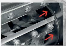
Rotary discs integral with the rotor and containment rings. Bench adjustment of rotating and fixed knives. Scissors cutting configuration.
